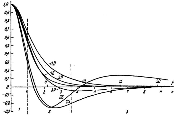
FIG. 2. Unnormalized functions  $x^{-l}R(x)$  for  $\mu$ -mesic lead ( $t = 2.279$ ): 1) solution in form of power series; 2) numerical integration; 3) asymptotic formulas;  $\rho = tx = Zr/a\mu$ .
