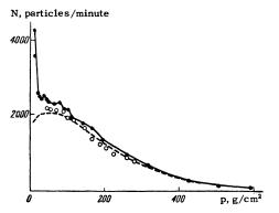
FIG. 1. Number of particles per minute as a function of the atmospheric pressure at the latitude of  $64^{\circ}$ N: • and 0 - results of measurements on July 8, 1958 during the ascent and descent of the apparatus respectively (time of start: 10 am Moscow time); dotted curve - average value of the number of particles obtained in measurements on July 1, 3 and 7, 1958.
