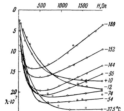
FIG. 5. Dependence of magnetostriction on temperature in the garnet ferrite  $3\text{Gd}_2\text{O}_3 \cdot 0.2 \text{Y}_2\text{O}_3 \cdot 4.8 \text{Fe}_2\text{O}_3$  (the figures on the curves show the temperature in degrees C).
