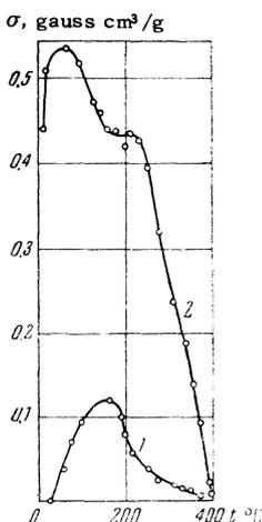
FIG. 10. Temperature dependence of the spontaneous magnetization of  $Gd_2O_3 \cdot Fe_2O_3$  in a magnetic field: 1) after first heating; 2) after second.
