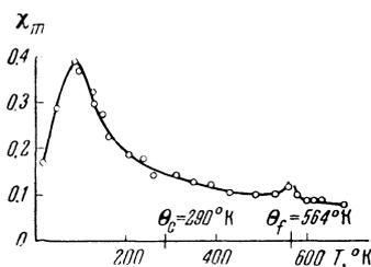
FIG. 4. Dependence of the paraprocess susceptibility on temperature in the garnet ferrite  $3\text{Gd}_2\text{O}_3 \cdot 5\text{Fe}_2\text{O}_3$ .
