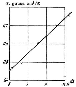
FIG. 7. Dependence of magnetization on  $H^{1/3}$  near the Curie point.
