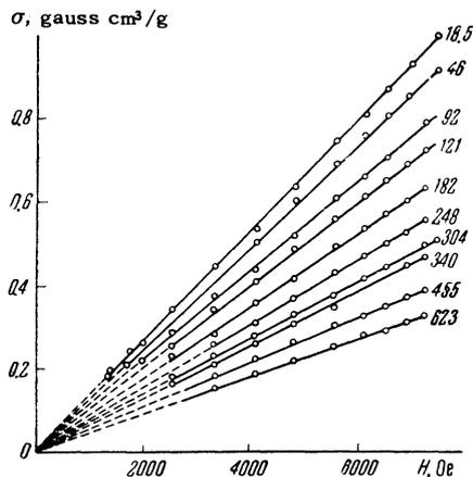
FIG. 11. Dependence of magnetization on field at various temperatures for  $Gd_2O_3 \cdot Mn_2O_3$  (the figures on the curves show the temperature in degrees C).
