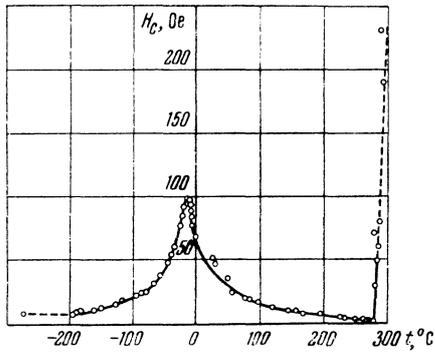
FIG. 3. Dependence of coercive force on temperature in the garnet ferrite  $3\text{Gd}_2\text{O}_3 \cdot 0.2 \text{Y}_2\text{O}_3 \cdot 4.8 \text{Fe}_2\text{O}_3$ .
