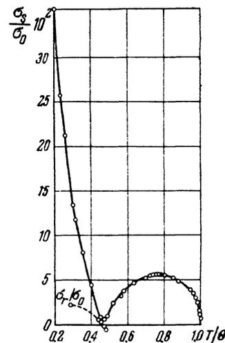
FIG. 2. Temperature dependence of  $\sigma_S/\sigma_0$  for the garnet ferrite studied. Dashed curve: temperature dependence of the residual magnetization  $\sigma_r/\sigma_0$  in the neighborhood of the compensation point.
