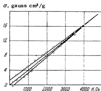
FIG. 12. Magnetic hysteresis in  $Gd_2O_3 \cdot Mn_2O_3$  at 4.3°K.
