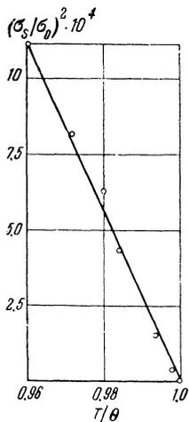
FIG. 6. Dependence of  $(\sigma_S/\sigma_0)^2$  on  $(T/\Theta)$  in garnet ferrite near the Curie point.
