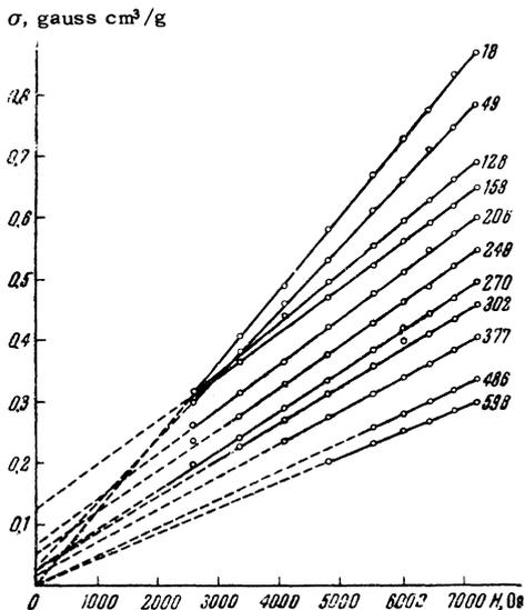
FIG. 8. Dependence of magnetization on field at various temperatures for gadolinium perovskite-ferrite,  $Gd_2O_3 \cdot Fe_2O_3$  (the figures on the curves indicate the temperature in degrees C).
