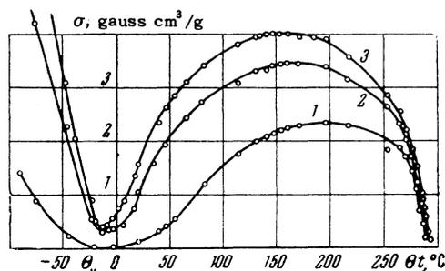
FIG. 1. Dependence of the specific magnetization on temperature at various fields in the garnet ferrite of composition  $3\text{Gd}_2\text{O}_3 \cdot 0.2\text{Y}_2\text{O}_3 \cdot 4.8\text{Fe}_2\text{O}_3$ : 1)  $H = 25.8$ ; 2)  $H = 129$ ; 3)  $H = 1550$  oe.
