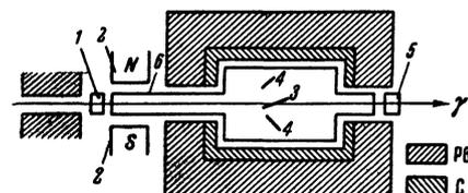
FIG. 1. Schematic diagram of the experimental setup. 1, 5 - ionization chambers, 2 - magnet, 3 - target, 4 - photographic plates, 6 - vacuum chamber.
