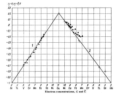
Curve 1-type A2 lattice; 2-type A1 and A3 lattices;  $\Delta$ -pure metals, × - Fe-Cr, •-Fe-V,  $\nabla$ -Fe-Ni, =-Co-Mn,  $\Box$ -Ni-Cr,  $\Delta$ -Ni-Mn, o-Fe-Co. sated spins) corresponding to this quantity, a change due to the fact that the outer portion of its electron shell (s and d) is substantially deformed in the crystalline state (compared with the shell of the isolated atom), is equal to\*
