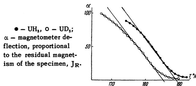
magnetism was produced by slowly cooling (for one hour) the specimens, placed in a magnetic field of approximately 200 oersteds, from room temperature to that of liquid nitrogen, after which the magnetic field was turned off and the specimen remained magnetized. The value of the residual magnetism depends, naturally, on the intensity of the magnetic field in which the specimen is cooled and on the lowest cooling temperature.
