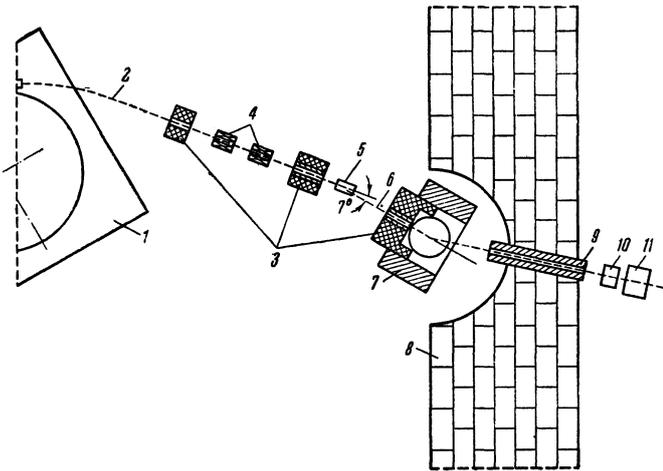
FIG. 1. Experimental setup. 1 – synchrocyclotron vacuum chamber, 2 – extracted proton beam, 3 – lead shield, 4 – quadrupole focusing lens, 5 – polyethylene target, 6 –  $\pi^+$  meson beam, 7 – deflecting electromagnet, 8 – cast-iron plates in the window of a concrete shield 4 meters thick, 9 – steel collimator, 10 – aluminum filter, 11 – propane bubble chamber.
