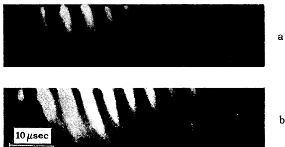
FIG. 3. High-speed photograph showing the motion of the plasma in air. The vertical scale is \Delta z = 11.5 cm along the z axis \tau = 280 \mu\text{sec} . a) U_c = 14.5 kv; b) U_c = 22.5 kv.
