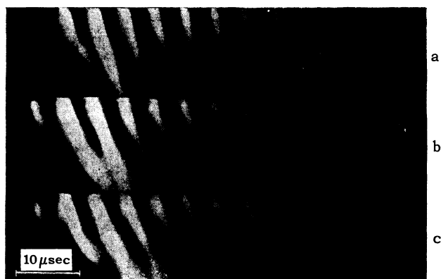
FIG. 4. High-speed photograph of the plasma pressure in helium along the z axis. \Delta z = 11.5 cm; U_c = 22.5 kv. a) \tau = 220 \mu\text{sec} , b) \tau = 280 \mu\text{sec} , c) \tau = 400 \mu\text{sec} .
