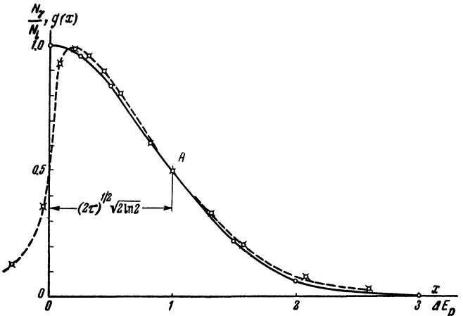
FIG. 4. Depth distribution of Si<sup>30</sup> ions in a tantalum backing. Solid line — theoretical distribution. The experimental points for target No. 1 are joined by dotted lines.
