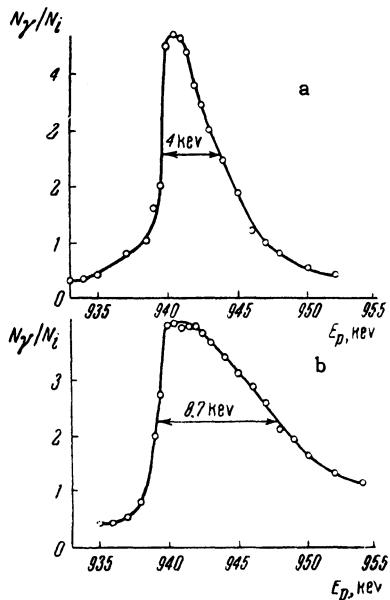
FIG. 2. Relative yield of gamma radiation from the Si<sup>30</sup>(p,  $\gamma$ ) reaction; resonance at  $E_p = 940$  kev, a) target No. 1 — Si<sup>30</sup> on tantalum backing; b) target No. 2 — Si<sup>30</sup> on copper backing. Ion energy  $E_i = 25$  kev.
