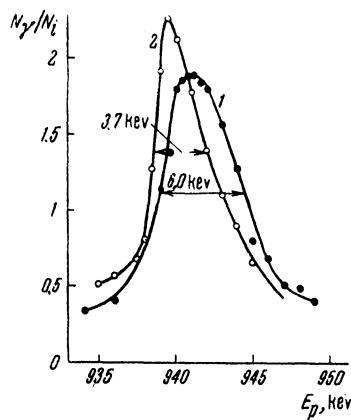
FIG. 3. Relative gamma yield in the Si<sup>30</sup>(p,  $\gamma$ ) reaction.
