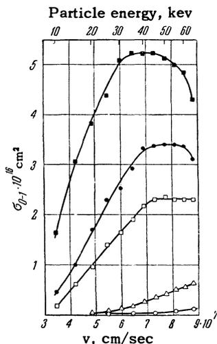
FIG. 3. Electron capture cross section for oxygen atoms in inert gases:  $\blacksquare$  Xe,  $\bullet$  Kr,  $\square$  Ar,  $\Delta$  Ne,  $\circ$  He.
