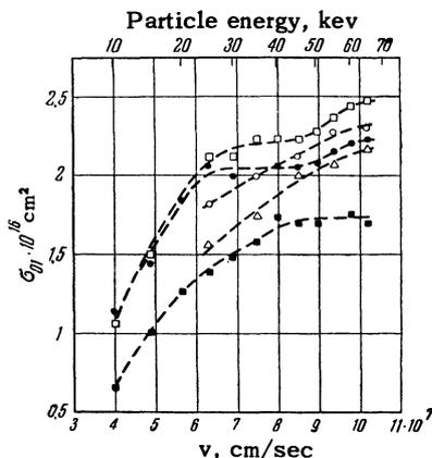
FIG. 5. Electron loss cross section for carbon atoms in inert gases:  $\blacksquare$  Xe,  $\bullet$  Kr,  $\square$  Ar,  $\Delta$  Ne,  $\circ$  He.
