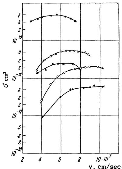
FIG. 9. Electron capture cross sections:  $\blacksquare$ )  $\sigma_{01}$ ,  $\blacktriangle$ )  $\sigma_{0-1}$ ,  $\bullet$ )  $\sigma_{1-1}$  for carbon;  $\triangle$ )  $\sigma_{0-1}$ ,  $\circ$ )  $\sigma_{1-1}$  for oxygen (in Xe).
