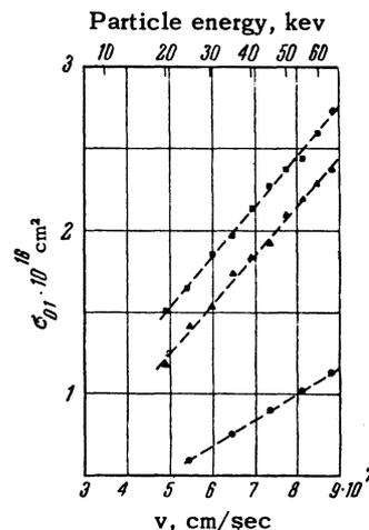
FIG. 8. Electron loss cross sections for oxygen atoms in molecular gases:  $\bullet$  H<sub>2</sub>,  $\blacktriangle$  N<sub>2</sub>,  $\blacksquare$  O<sub>2</sub>.
