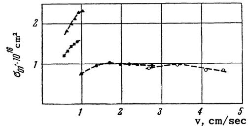
FIG. 13. Electron loss cross sections for fast atoms:  $\blacktriangle$  C,  $\blacksquare$  O,  $\bullet$  H,  $\circ$  He (in He).
