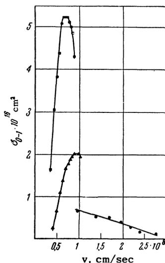
FIG. 10. Cross sections for the capture of one electron in atoms:  $\blacksquare$ ) O,  $\blacktriangle$ ) C,  $\bullet$ ) H (in Xe).
