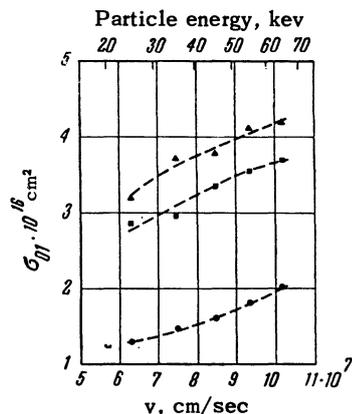
FIG. 6. Electron loss cross sections for carbon atoms in molecular gases:  $\bullet$  H<sub>2</sub>,  $\blacktriangle$  N<sub>2</sub>,  $\blacksquare$  O<sub>2</sub>.
