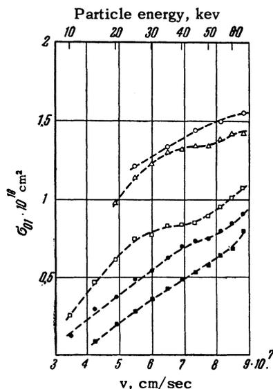
FIG. 7. Electron loss cross section for oxygen atoms in inert gases:  $\blacksquare$  Xe,  $\bullet$  Kr,  $\square$  Ar,  $\Delta$  Ne,  $\circ$  He.
