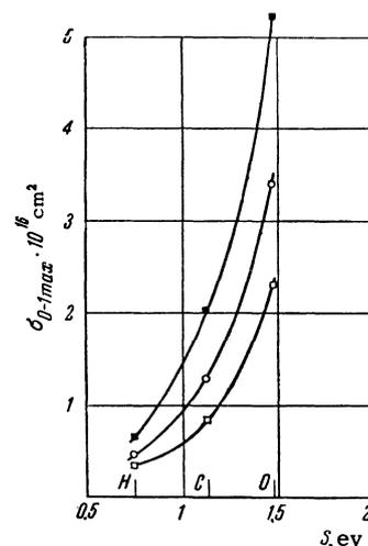
FIG. 11. The dependence of  $\sigma_{0-1 \max}$  on electron affinity:  $\square$ ) Ar,  $\circ$ ) Kr,  $\blacktriangle$ ) Xe.
