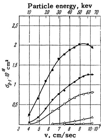
FIG. 1. Electron capture cross sections for carbon atoms in inert gases:  $\blacksquare$  Xe,  $\bullet$  Kr,  $\square$  Ar,  $\Delta$  Ne,  $\circ$  He.
