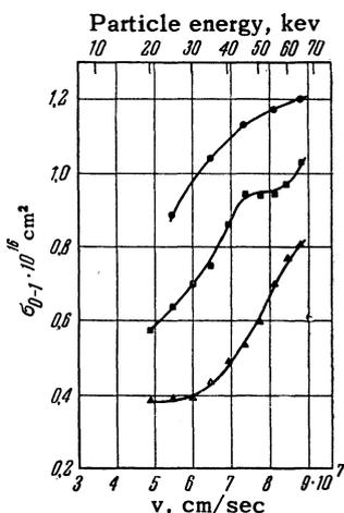
FIG. 4. Electron capture cross section for oxygen atoms in molecular gases:  $\bullet$  H<sub>2</sub>,  $\Delta$  N<sub>2</sub>,  $\blacksquare$  O<sub>2</sub>.
