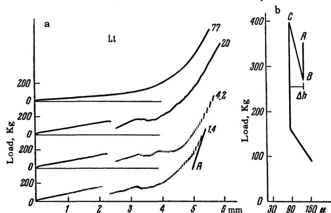
FIG. 1. a - Machine compression diagrams for specimens of chemically pure lithium at temperatures from 77 to  $1.4^\circ\text{K}$ ; b - Dilatometric curve taken during warming of the lithium specimen deformed at a temperature of  $1.4^\circ\text{K}$ .
