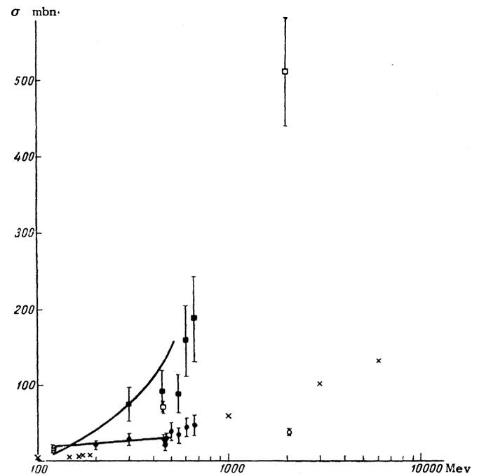
FIG. 3. Dependence of the tritium production cross section of aluminum, lead and iron on proton energy. ■, □ - Pb; ●, ○ - Al; × - Fe; solid curve - calculation by evaporation theory.
