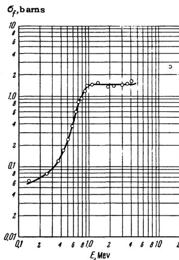
The  $Pu^{240}$  fission cross section is  $1.50 \pm 0.15$  barns at the plateau and agrees with the results obtained by Dorofeev and Dobrynin<sup>1</sup> by measurements with neutrons from a Ra-Be source ( $1.40 \pm 0.15$  barns). The fission cross section obtained for 15-Mev neutrons was  $2.6 \pm 0.2$  barns.
