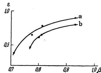
FIG. 2. Dependence of the Cerenkov-counter efficiency  $\epsilon$  on the velocity of detected particles  $\beta$ . a - plexiglass, b - water.
