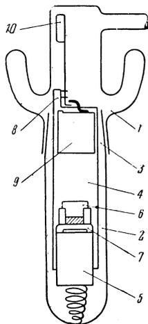
(see diagram). The upper portion of the instrument consisted of a trap 1 for the lubricant vapor with a ground neck. The lower portion of the instrument consists of a sealed tube 2 which was inserted into ground section 3. Placed inside the instrument was a setup for cleaving solid specimens to incandescence, consisting of stainless steel tube 4 with windows, and of a brass cylinder with spring 5. Attached to this cylinder were guides for a knife 6
