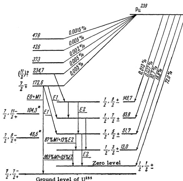
FIG. 4. Low-lying excited levels of  $\text{U}^{235}$  (from  $\alpha$  decay data in Ref. 3). \* - marks levels known from the Coulomb excitation of  $\text{U}^{235}$ . The energies of all levels are expressed in kev and computed from the "zero level."
