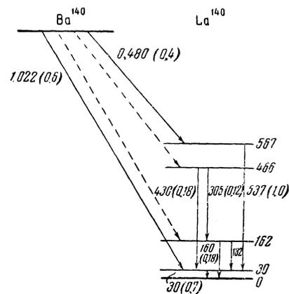
FIG. 4. Decay scheme of  $Ba^{140}$ .
