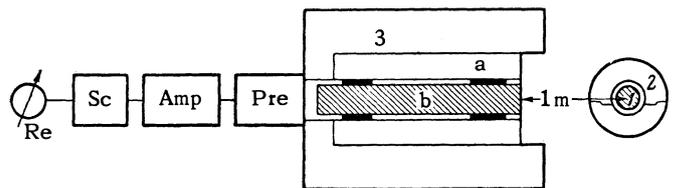
FIG. 1. Arrangement of the experiment. 1 - neutron source, 2 - absorbing sphere of sample material, 3 - long counter: a - paraffin container, b - boron counter; Pre - preamplifier, Amp - amplifier, Sc - scaler, Re - mechanical recorder.
