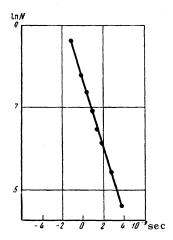
mined the lifetime of the 264-kev level of  $\mathrm{Er}^{167}$ . The figure gives on a semilogarithmic scale the decay curve of the state under investigation (the delay time is plotted along the horizontal axis) from which the half-life is found to be
