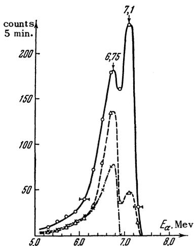
FIG. 2. Spectrum of  $\alpha$ -particles in the californium fraction at various times. (Solid curve) — 1 hr. 33 min. after the end of bombardment; (dashed curve) — 3 hrs. 23 min. after the end of bombardment; (dot-dashed curve) — 24 hrs. 49 min. after the end of bombardment.
