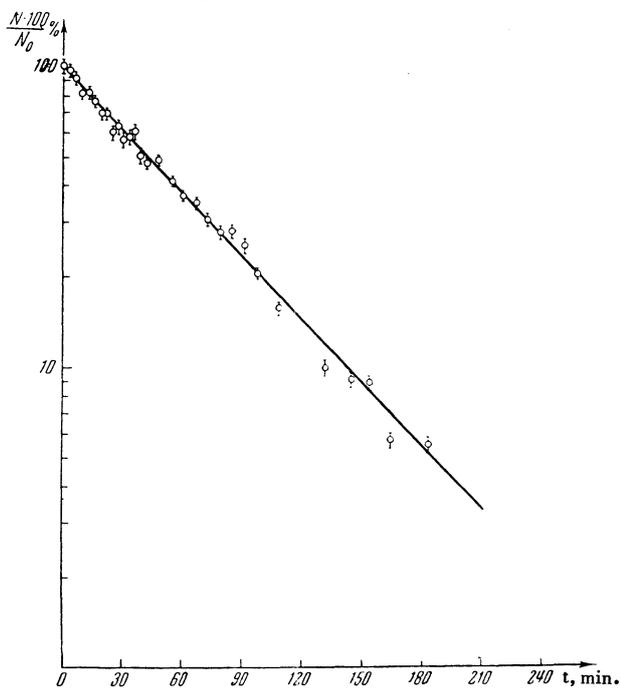
FIG. 4. Decay curve of Cf<sup>245</sup>.  $T_{1/2} = 44$  min.
