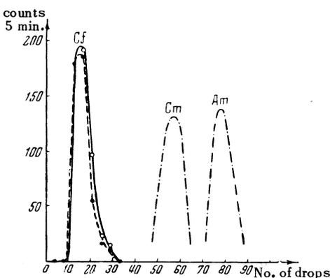
FIG. 1. Elution curves from the chromatographic separation. Solid dots (dashed curve) —  $\text{Cf}^{246}$ , open points (solid curve) —  $\text{Cf}^{245}$ .
