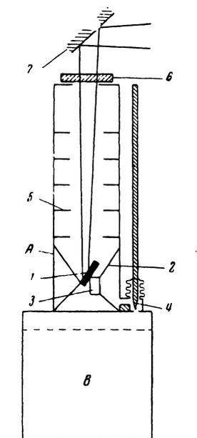
FIG. 1. (A) vacuum calorimeter, (B) carbon "pump," (1) sample, (2) caprone rods, (3) bronze thermometer, (4) valve for carbon "pump," (5) diaphragms, (6) window of KRS-5, (7) mirror.
