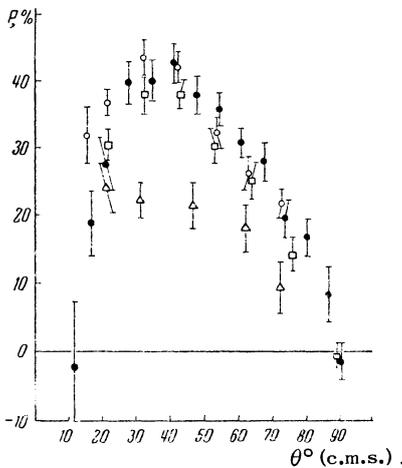
FIG. 2. Dependence of the polarization  $P_H(\theta)$  in elastic p-p scattering on the angle of scattering: ● - present work, ○ - 415 Mev,<sup>15</sup> □ - 315 Mev,<sup>12</sup> Δ - 170 Mev.<sup>16</sup>
