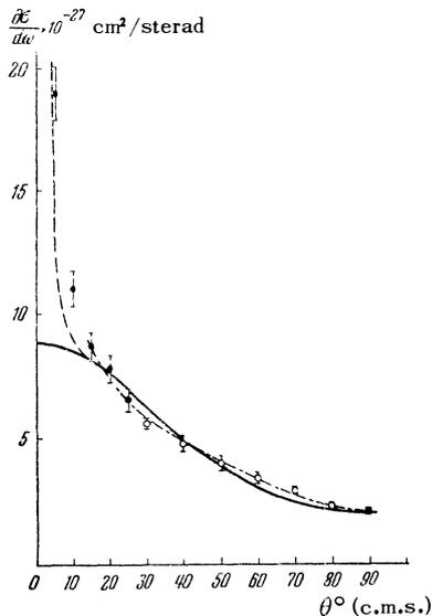
FIG. 3. Dependence of the cross-section for elastic p-p scattering at 657 Mev on the angle of scattering from the following sources: ●—Ref. 10, ○—Ref. 8, ■—average of results from (8) and (9); the solid curve corresponds to formula (5); the dashed curve gives the sum  $\sigma_N(\theta) + \sigma_C(\theta)$ ; the dot-dashed curve has been drawn through the points visually.
