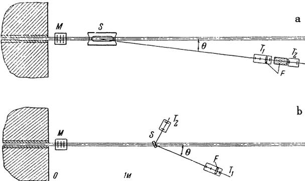
FIG. 1. Experimental setup. M—Monitor, S—Scatterer, T<sub>1</sub>, T<sub>2</sub>—telescopes, F—copper absorber.
