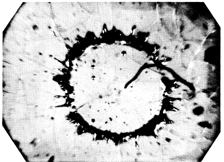
FIG. 7. Microphotograph of the deposit on a vitreous target obtained during the explosion of an 0.07 mm iron wire. Amplification 130 \times .
