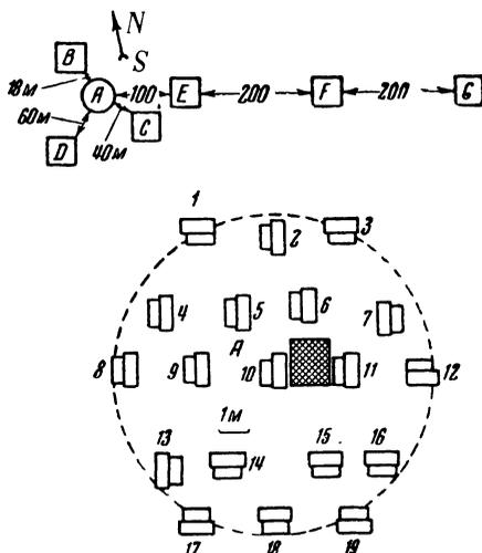
FIG. 1. Experimental arrangement for measuring the particle current density in extensive atmospheric showers whose axes fall near point A. The small arrow near B points north. The crosshatched rectangle near A denotes a detector for penetrating particles.
