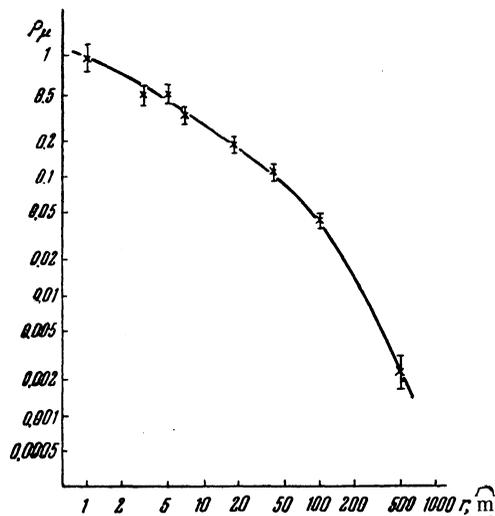
FIG. 3.  $\mu$  meson current density (for mesons with energy  $\geq 440$  Mev) vs. distance from the shower core.
