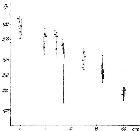
FIG. 4. Spatial distribution of  $\mu$  mesons with energy more than 440 Mev in extensive showers with various (total) numbers of particles:  $\times$ — $0.53 \times 10^5$ ;  $\Delta$ — $1.5 \times 10^5$ ;  $\circ$ — $3.2 \times 10^5$ ;  $\bullet$ — $10^6$ . The  $\mu$  meson current density is normalized relative to showers with  $2 \times 10^5$  particles, using the number of  $\mu$  mesons 100 m from the axis of the shower.
