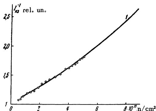
FIG. 3.  $1 - s = 300$  cm/sec;  $\theta = 1.1 \times 10^{-15} \text{ cm}^2$ ;  $\circ$  — experimental points. The ordinate is labeled  $I_{sc}^{-1}$  (relative units) and the abscissa is labeled neutrons/cm<sup>2</sup>.
