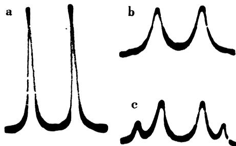
FIG. 1. Twin resonance absorption in the free radical of *aa*-diphenyl- $\beta$ -trinitrophenyl-hydrazyl at  $\nu = 30$  Mc and  $T = 300^\circ\text{K}$ . a)  $\alpha = 90^\circ$  with field ( $H_\nu \approx 0.1$  oersted) b)  $\alpha = 90^\circ$  and c)  $\alpha = 45^\circ$  with strong field ( $H_\nu = 2$  oersteds)
