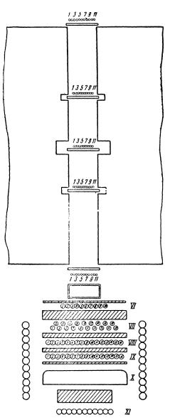
FIG. 1. Distribution of the counters in the telescope and of the absorbers.
