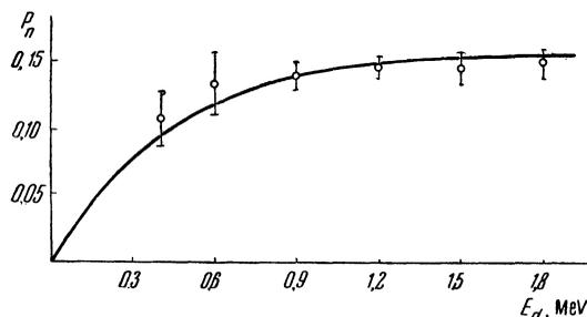
FIG. 1. "Exit" polarization of (D + D) neutrons for angle  $\theta_n$  (lab) =  $49^\circ$  obtained from measurements using a thick target for various deuteron energies  $E_d$ .
