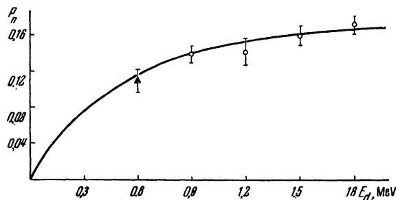
FIG. 2. Polarization of (D + D) neutrons at angle  $\theta_n$  (lab) =  $49^\circ$  obtained from measurements with a thick target for various deuteron energies  $E_d$ .  $\Delta$ : results of measurements by Meier, Scherrer and Trumpy<sup>2</sup>.
