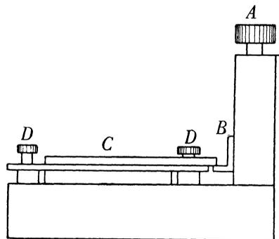
FIG. 3. Diagram of fixture for separating the optical contact. *A*—knob of lifting screw, *B*—hook used to separate the glass plate, *C*—glass plate, *D*—clamping screws.
