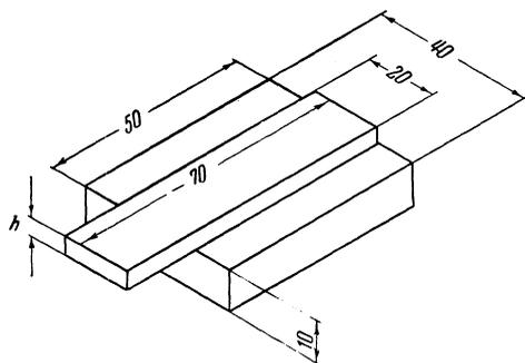
FIG. 2. Sketch of glass plates, placed in optical contact;  $h = 0.5, 1.0,$  and  $2.0$  mm. All dimensions are given in millimeters.
