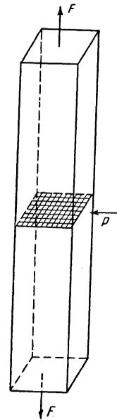
FIG. 1. Glass bars, placed in optical contact.  $FF$ —tension force,  $P$ —surface of optical contact.
