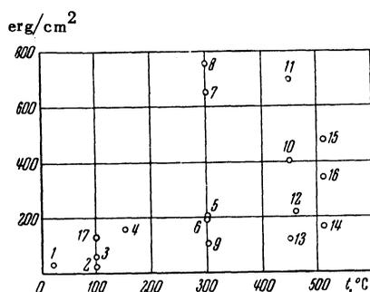
FIG. 6. Work of separation of optical contact as a function of the sintering temperature.
