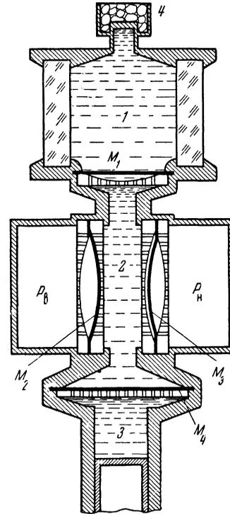
A schematic plan of the set-up is given in the Figure. It consists of the chamber 1, a limiter 2, and compressor 3. The chamber 1 has a cylindrical form and is filled with freon-13 ( $\text{CClF}_3$ ). The volume of the chamber is 1 liter. The viewing windows are discs of organic glass mounted without gaskets. The membrane  $M_1$  is constructed out of rubber made from domestic synthetic nayrite.
