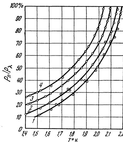
FIG. 1. Dependence of  $\rho_n / \rho_\lambda$  upon temperature: 1—pure He<sup>4</sup>; 2—3.0% He<sup>3</sup>; 3—5.6% He<sup>3</sup>; 4—8.2% He<sup>3</sup>
