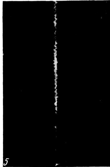
FIG. 5. Wire 150 mm long, 0.15 mm dia.  $U_0 = 4$  kv. Capacitor 10 microfarad.
