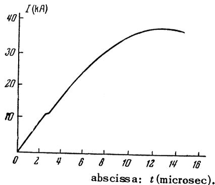
FIG. 12. Oscillogram of current for wire explosion in vacuum. Wire 45 mm long, 0.15 mm dia,  $U_0 = 25$  kv.
