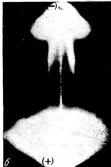
FIG. 6. Wire 45 mm long, 0.15 dia.  $U_0 = 20$  kv.
