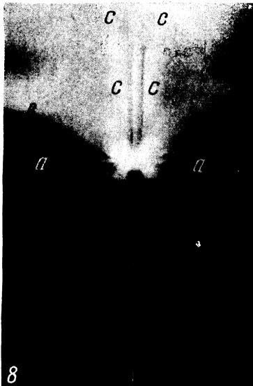
FIG. 8. Wire 90 mm long, 0.15 mm dia,  $U_0 = 35$  kv. A plexiglass plate measuring  $1 \times 100 \times 100$  mm was placed transverse to the wire.
