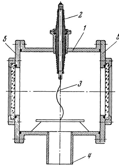
FIG. 1. Diagram of a vacuum chamber.
