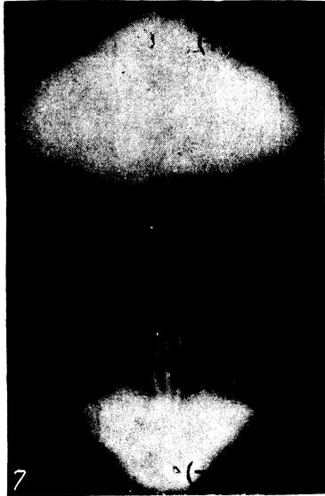
FIG. 7. Wire 45 mm long, 0.15 mm dia,  $U_0 = 30$  kv.
