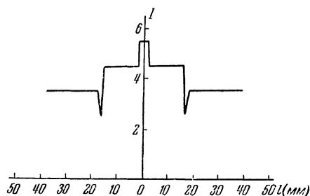
FIG. 11. Photometry curve of copper deposited on insulating plate. *I*—intensity of light in relative units, *l*—distance from center of hole in plate.
