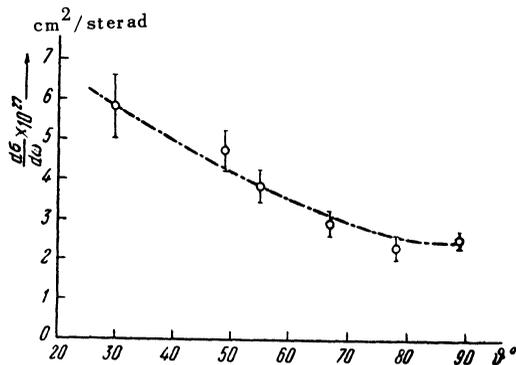
FIG. 3. Differential cross section for elastic scattering of neutrons by neutrons at 590 mev. Curve— $\sigma_{pp}(\vartheta)$  at  $E_p = 590$  mev<sup>14</sup>; Points— $\sigma_{nn}(\vartheta)$  for  $E_n = 590$  mev.
