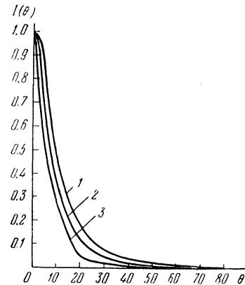
FIG. 1. Calculated values of the integral  $I(\theta)$  for various neutron energies: 1—300, 2—450, 3—600 mev.
