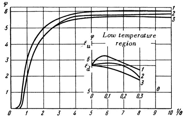
FIG. 2. Dependence of the position of the Fermi level on the temperature. 1— $N_d = 7.5 \times 10^{15} \text{ cm}^{-3}$ ,  $N_a = 7.5 \times 10^{10} \text{ cm}^{-3}$ ; 2— $N_d = 7.5 \times 10^{14} \text{ cm}^{-3}$ ,  $N_a = 7.5 \times 10^{13} \text{ cm}^{-3}$ ; 3— $N_d = 7.5 \times 10^{15} \text{ cm}^{-3}$ ,  $N_a = 6.75 \times 10^{15} \text{ cm}^{-3}$
