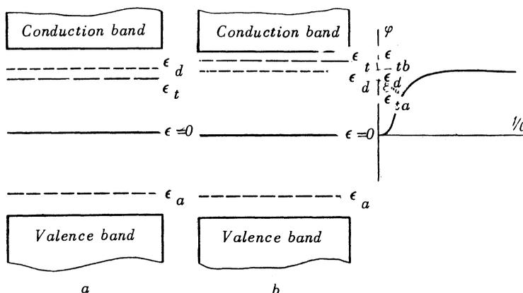
FIG. 5. Energy diagram of *n*-type germanium for  $\epsilon_t > 0$ . On the right-hand side of the diagram is shown the dependence on the temperature of the Fermi level, with the energies of the traps in both cases *a* and *b* indicated on the vertical axis.
