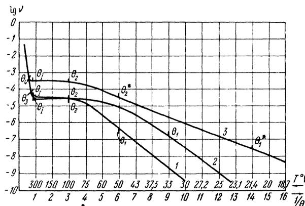
FIG. 3. Temperature dependence of the density of charge carriers. 1-  $N_d = 7.5 \times 10^{15} \text{ cm}^{-3}$ ,  $N_a = 6.75 \times 10^{15} \text{ cm}^{-3}$ ; 2-  $N_d = 7.5 \times 10^{14} \text{ cm}^{-3}$ ,  $N_a = 7.5 \times 10^{13} \text{ cm}^{-3}$ ; 3-  $N_d = 7.5 \times 10^{15} \text{ cm}^{-3}$ ,  $N_a = 6.75 \times 10^{10} \text{ cm}^{-3}$ .
