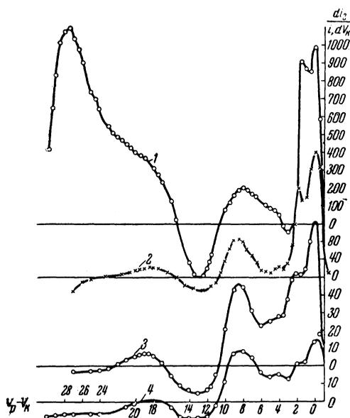
FIG. 1. The distribution curves of the electrons reflected according to (their) energies are obtained from the four values  $V_p$ : 1–30, 2–75, 3–150, 4–260 v. The maximum of curve 1 when  $V_p - V_k = 27$  v is dependent on the true secondary electrons.
