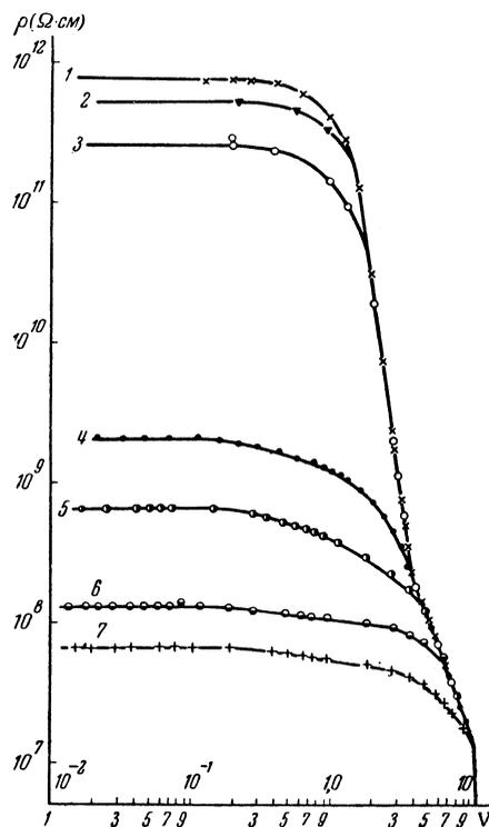
FIG. 2.  $\rho$  ( $\Omega \cdot \text{cm}$ ) vs.  $V$ . The dependence of the resistance on the external electrical field: (v/cm): 1--0.15; 2--0.2; 3--0.4; 4--1.77; 5--2.23; 6--3.12; 7--4.2° K; ( $V_{cr} = 11$  v/cm).
