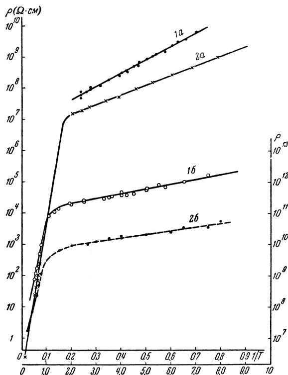
FIG. 1.  $\rho$  (ohm-cm) vs.  $1/T$  (left scale),  $\rho$  vs  $1/T$  (right scale). The dependence of resistance on the temperature: 1a, 2a, in the region of hydrogen and helium temperatures (left scale), 1b, 2b, in the region of helium and very low temperatures (right scale).
