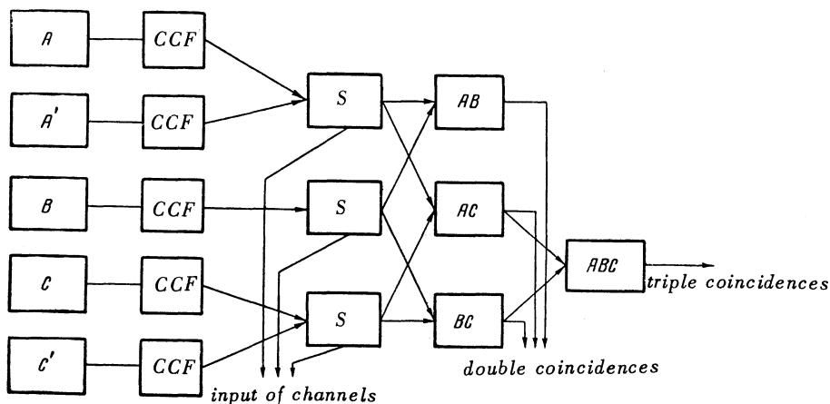
FIG. 2. Block diagram of the detection system:  $A$ ,  $A'$ ,  $B$ ,  $C$  and  $C'$  -- scintillation counters (same symbols as in Fig. 1);  $CCF$  -- cascade cathode follower;  $S$  -- pulse shaping circuit;  $AB$ ,  $AC$  and  $BC$  -- double coincidence circuits,  $ABC$  -- triple coincidence circuit.
