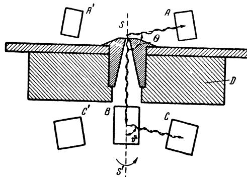
FIG. 1. Principal view of the apparatus:  $SS'$  — symmetry axis of the instrument,  $S$  — the source,  $A$  and  $A'$  — scintillation crystals of detectors insensitive to the polarization of photons,  $B$  — the central crystal of polarimeter,  $C$  and  $C'$  — side crystals of polarimeter,  $D$  — the shield.
