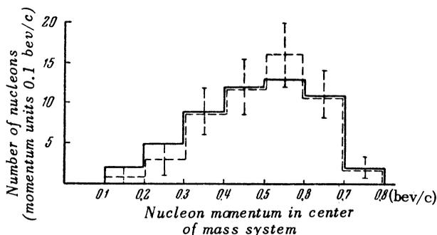
FIG. 2. Nucleon momentum distribution in the center of mass system for the reactions  $(p-0)$  and  $(n+-)$ . Dashed line— Eisberg et al., experimental distribution; solid line— distribution according to the statistical theory including isobar states.
