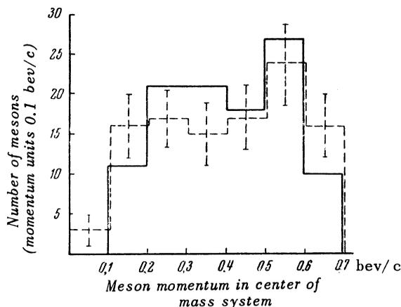
FIG. 1. Meson momentum distribution in the center of mass system for the reactions  $(p-0)$  and  $(n+-)$ . Dashed line — Eisberg et al, experimental distribution; solid line— distribution according to the statistical theory including isobars.
