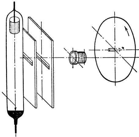
FIG. 3. Diagram for the observation of arc propagation.
