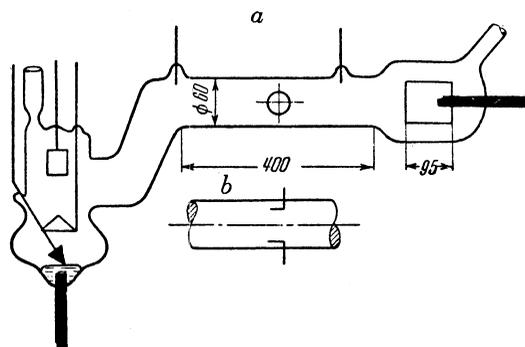
FIG. 1. a--mercury tube, b--arrangement of the two symmetrical probes with respect to the axis of the tube.
