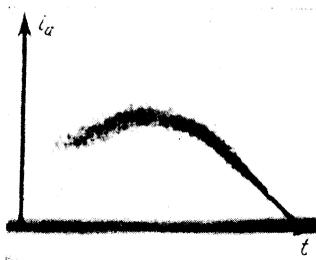
FIG. 11. Oscillogram of the arc current in Hg vapor at  $R = 30$  mm,  $(i_a)_{\max} = 2000$  amp,  $p = 0.8 \mu\text{Hg}$ .
