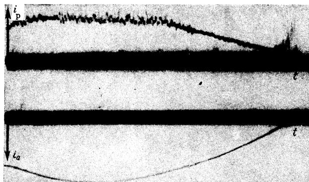
FIG. 10. Probe current  $i_p$  and arc current  $i_a$ , Ar,  $R = 30$  mm,  $(i_a)_{\max} = 240$  amp,  $p = 3 \mu\text{Hg}$ .
