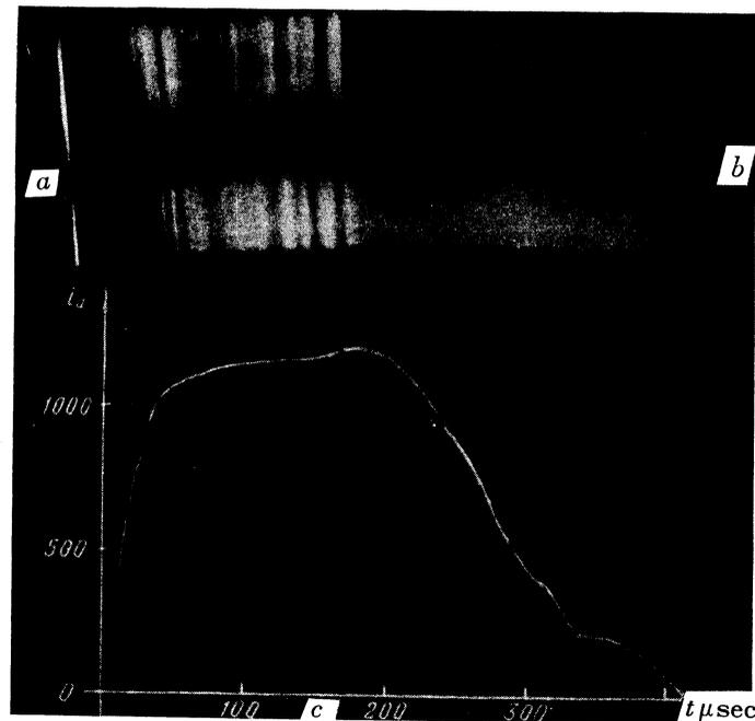
FIG. 21. *a*--photograph of the narrow band of the arc on a stationary film, *b*--the same on a moving film, *c*--oscillogram of the current.
