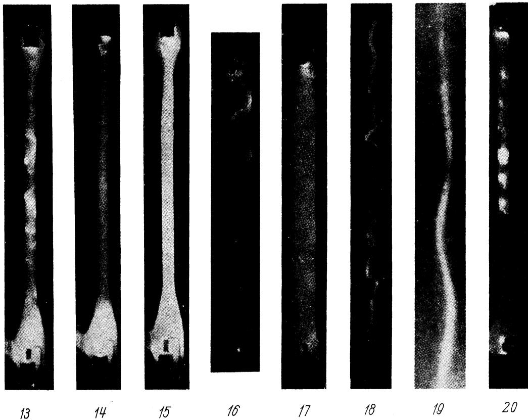
FIG. 13. The arc at a current pulse of 450 amp,  $\tau = 2 \mu \text{ sec}$ , Hg,  $R = 5 \text{ mm}$ ,  $p = 1 \mu \text{ Hg}$ .
