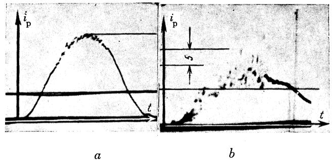
FIG. 7. Probe current at  $(i_a)_{\text{max}} = 1700 \text{ amp}$ ,  $p = 1 \mu\text{Hg}$ . a--at the axis of the tube, b--at the walls.
