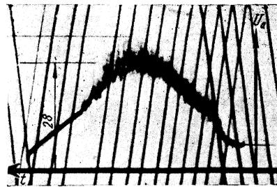
FIG. 6. Arc voltage at  $(i_a)_{\text{max}} = 1700 \text{ amp}$ ,  $p = 0.4 \mu\text{Hg}$ .
