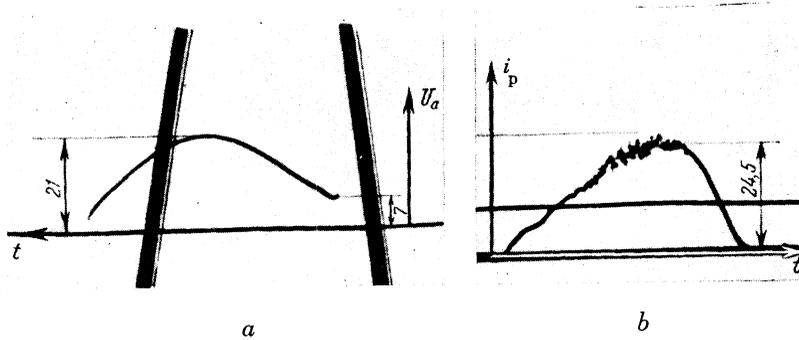
FIG. 9. Arc voltage and probe current at  $(i_a)_{\max}$
