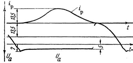
FIG. 5. The arc voltage  $U_a$  and the ionic current in the probe  $i_p$  when  $(i_a)_{\text{max}} = 1.0 \text{ amp}$ ,  $p = 0.4 \mu\text{Hg}$ .
