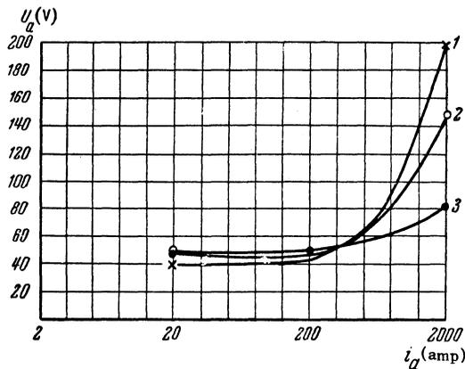
FIG. 4. The dependence of the arc voltage on the current in a cylindrical tube. 1-- $p = 1$ , 2-- $p = 10$ , 3-- $p = 100 \mu\text{Hg}$ .
