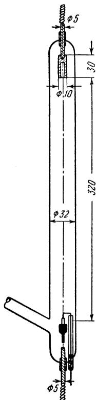
FIG. 2. Tube used in the experiments with  $H_2$  and with inert gases.
