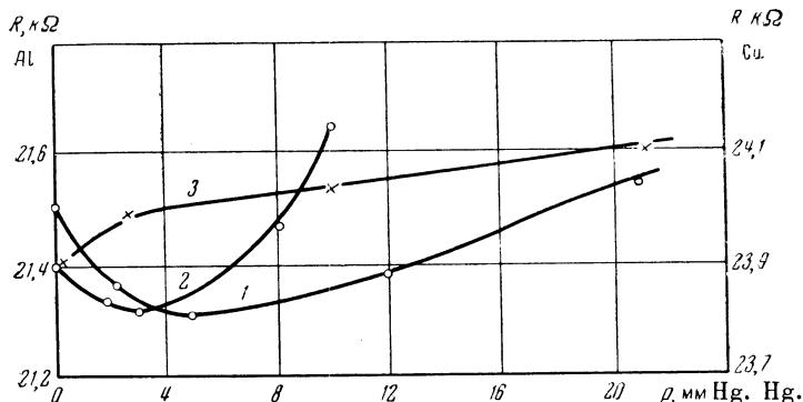
FIG. 1. Change of metal-to-semiconductor contact resistance with air pressure: 1 and 2 — copper oxide — aluminum ( $V_k = 1.18$  v), two samples; 3 — copper oxide — copper ( $V_k = 0.22$  v).
