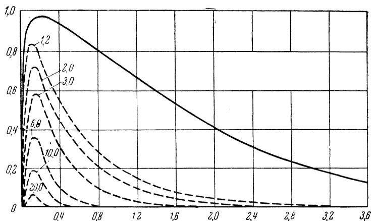
FIG. 2. The solid curves show the dependence of the number of true fissions ( $Q_1M^{-1}$ ), and the broken lines, the dependence of the number of false fissions, associated with the superposition of  $\alpha$ -particles pulses ( $Q_2N^{-1}$ ) on the potential  $V$  of the discriminator (horizontal axis) for different values of  $\alpha$ , shown on the curves, in the case  $M\tau = 10^{-4}$ ,  $N\tau = 10^{-3}$ . The potential is in units of  $b^{-1}$
