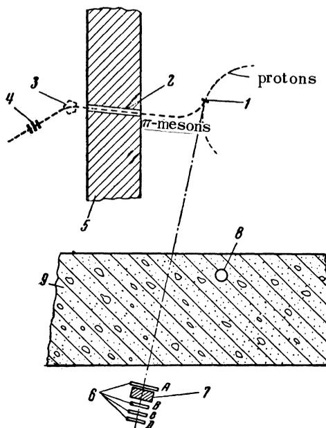
Experimental Arrangement. 1-target; 2-collimator; 3-deflecting magnet; 4-telescope of scintillator detectors, used as a monitor; 5-iron shield; 6-telescope of proportional counters, serving as a "detector of penetrating radiation"; 7-converter; 8-counter, filled with BF<sub>3</sub>; 9-concrete shield.
