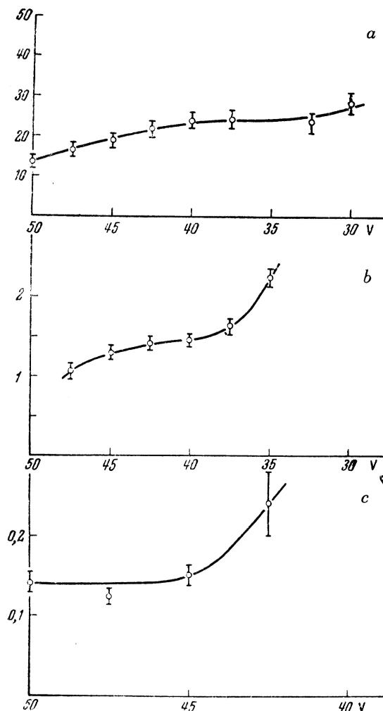
FIG. 2. Dependence of the relative fission counting rate on discriminator locking potential for a - uranium, b - bismuth and c - wolfram.
