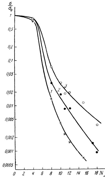
FIG. 6. Dependence of the fission cross section of nuclei on the minimum number of neutrons which must be emitted before fission (assuming that one proton is also emitted). 1 -  $E_n = 84$  mev; 2 -  $E_n = 120$  mev; 3 -  $E_n = 380$  mev.
