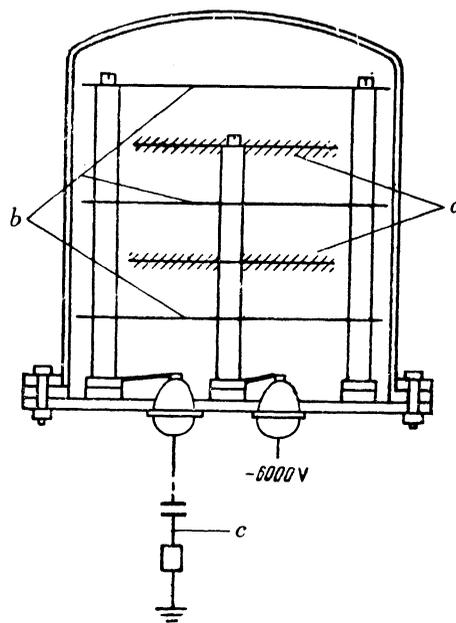
FIG. 1. Drawing of the ionization fission fragment chamber. *a* - the fissioning material; *b* - collecting electrodes; *c* - to amplifier grid.
