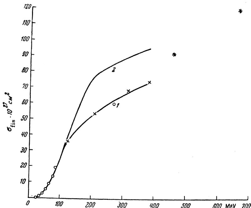
FIG. 3. Dependence of fission cross section of bismuth on neutron energy. 1 - without corrections for the energy spectrum of the incident neutrons; 2 - with such correction. The stars indicate data on the fission of bismuth by protons<sup>23</sup>.
