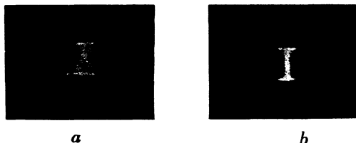
FIG. 11. Discharge in argon: a : un-filamented discharge, p = 200 mm mercury; b : filamented discharge, p = 300 mm mercury.
