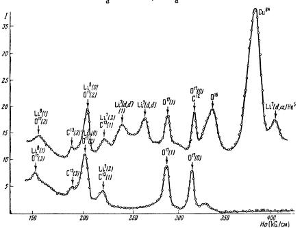
FIG. 2. The energy spectrum of lithium.  $E_d = 3.76$  mev. Microphotogram of the half plate: above - irradiated without the filter; below - irradiated with the filter.
