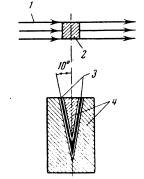
Fig. 1. Experimental arrangement 1. Proton beam. 2. Target. 3. Photographic plate. 4. Brass block.
