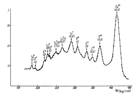
FIG. 3. The energy spectrum of lithium.  $E_d = 4.69$  mev. Microphotogram of the half plate irradiated without the filter.
