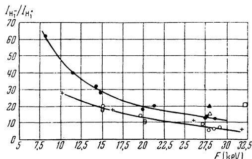
FIG. 4. Value of  $I_{H_1^-} / I_{H_1^+}$  for a beam of  $H_1^+$  passing through: ○ = Al-foil; ● = Be-foil; + = Cu-foil. Values for  $I_{D^+}$  for a beam of  $D^+$ , passing through:  $\Delta$  = Al-foil;  $\blacktriangle$  = Be-foil; Value of  $I_{H_2^-} / I_{H_2^+}$  for  $H_2^+$  beam passing through: □ = Al-foil.
