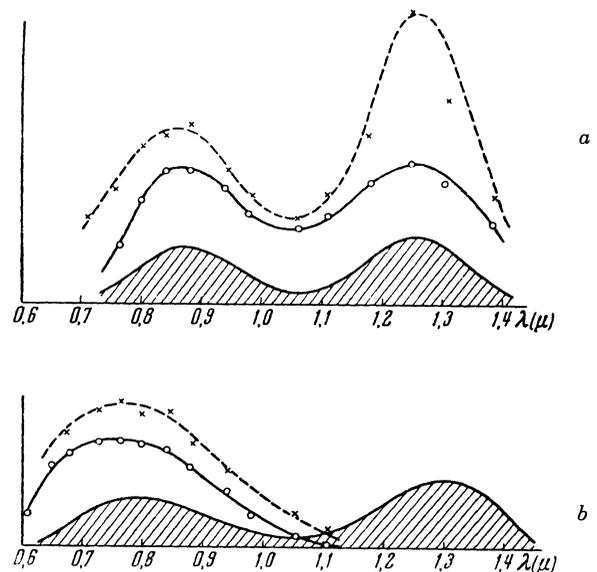
a. ZnS-Cu, Tu-phosphor, b. ZnS·CdS-Cu, Ni-phosphor. Continuous lines --- dielectric constant, dotted lines --- intensity of excitation.
