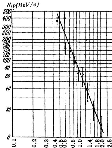
Fig. 3. Pulse spectrum of protons produced by neutrons in lead of thickness 11.3 gm/cm<sup>2</sup>.
